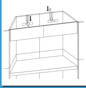
ALCOVE CEILING PANEL INSTALLATION: Hang ceiling panel brackets from top of backwall.
